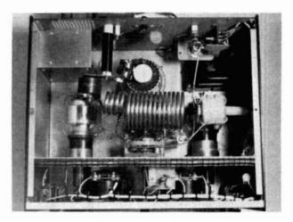
Top view of amplifier illustrates small size of 3CX1200A7. Compare it to the vacuum variables in the lower section of the photo.
